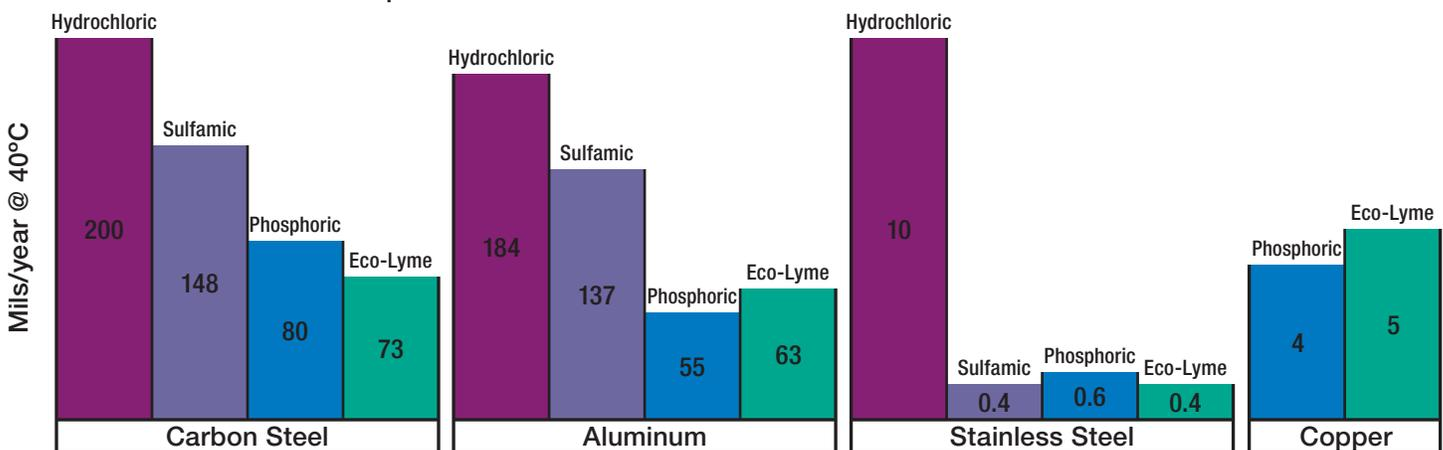
Test Conditions: Coupons immersed for seven days, static conditions, 100 mL closed vessel per ASTM methods.
