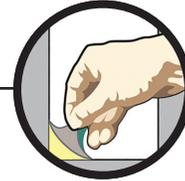
5. Remove the film backing on the top side to expose to UV light or sunlight.
