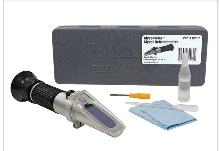
The reading should be at or close to the 32° line. If it is not at 32°, use the included screwdriver to adjust the calibration screw (under the rubber boot) until the blue line is at 32°.
