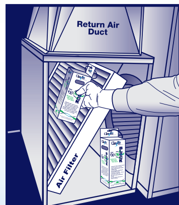
Shown are two typical Odor-Block placements in an HVAC system.
