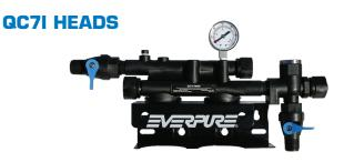
Used with any Everpure filters. All sizes come with a built-in shut off, flushing valve and an outlet pressure gauge which is included on the mounting bracket. (3/8 NPT)
