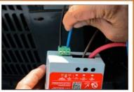
Attach the blue wire (supplied) to the Start Winding on the NuStart green terminal connector.
